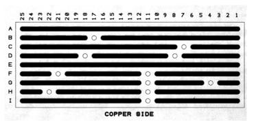
2. The next stage is to insert the terminals, wire links and components. Do not touch the copper tracks with fingers, they must be kept clean and grease free until all soldering is completed. Trim the leads and solder them into position in a methodical order as recommended below.
